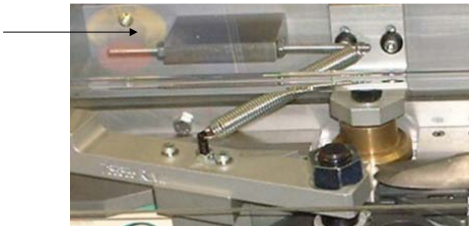
Figure 25. Doming Wheels Adjustment
